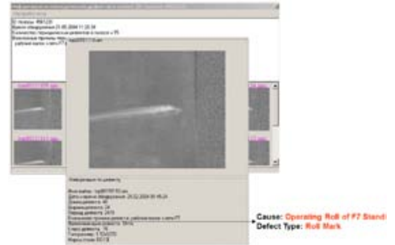
Figure 4 - Visualization of application of processing of periodical defects
