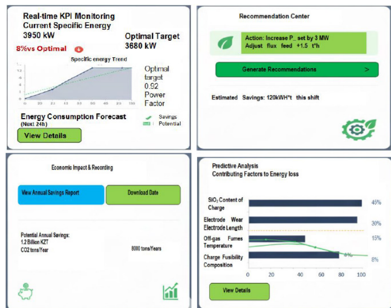
Figure 5 – Energy consumption optimization management platform of a metallurgical enterprise
