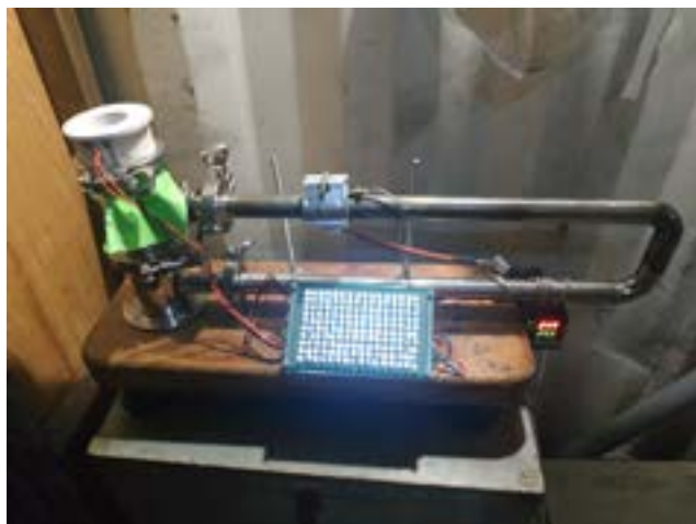
Figure 2 – Laboratory sample of a single-stage TAD
