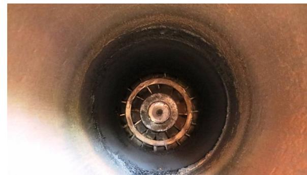
Figure 3 – Swirlers inside the combustion chamber
