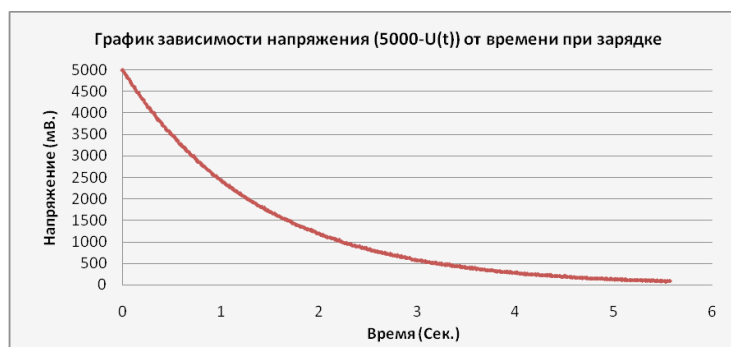
Figure 14 – The graph of voltage versus time for charging C1 through R1
