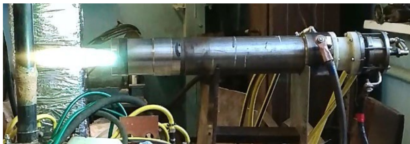
Figure 5 – Photograph of the plasma torch in operation
